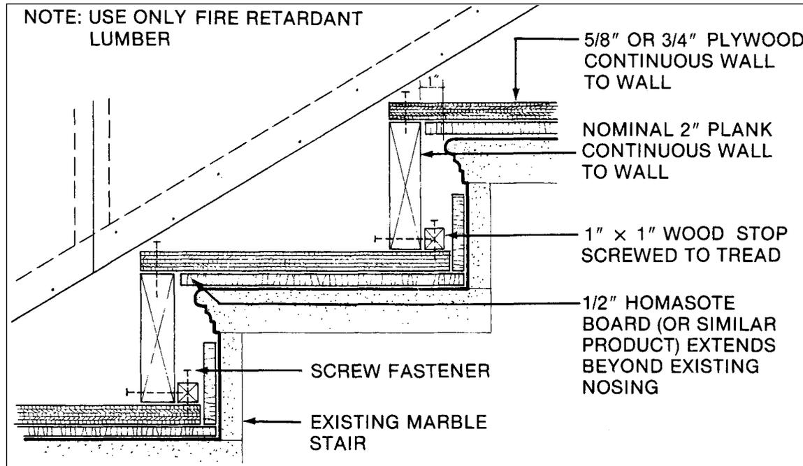
*Historic features that characterize a building should always be protected from damage during rehabilitation work. The drawing shows how a resilient, temporary stair covering was applied over the existing marble staircase. Drawing: National Park Service staff, based on material originally prepared by Emery Roth and Sons, P.C.*
